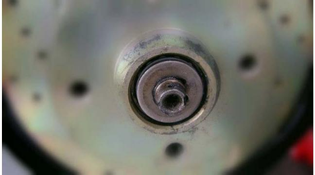
Wind on the 24mm nut. You need to tighten it up and then back the nut off slightly so the disk turns nicely.
