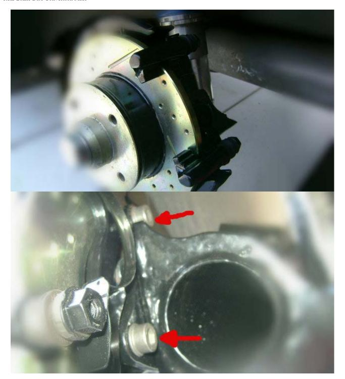
Time to fit the pads. So start by copper greasing the carrier for the pads to slide on. I have pointed out the outside sliders bud you must do the slides for the inside pad too.
