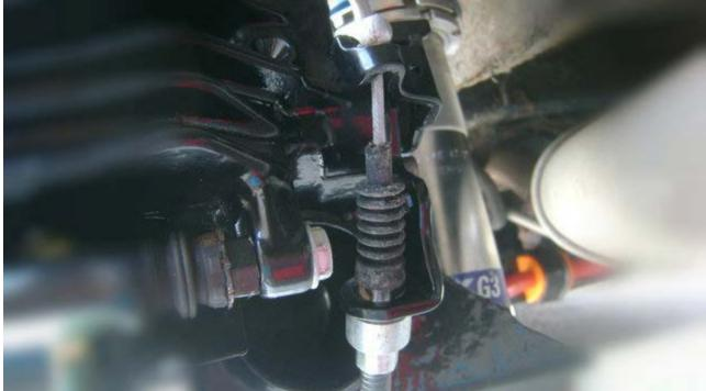
Now this is where i am confused. I had heard you need to cut 10mm off the sleeve to give you enough length for the cable to reach the handbrake inside the car. I didn't need to but i have provided a picture in case you do.
