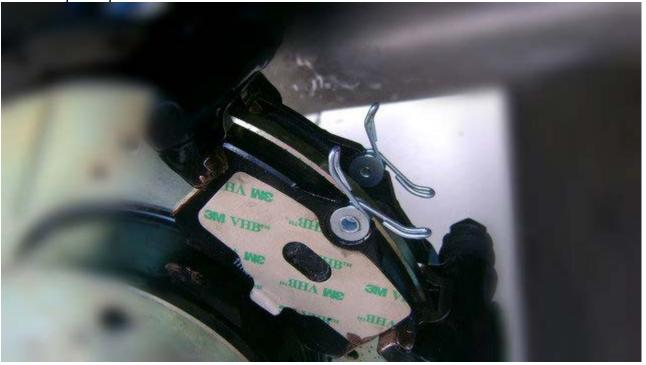
You can now fit the caliper. Ensure you have wound the piston back in or you will struggle to get it over the new pads and disks (if used). You need to fit the caliper so the handbrake mount is at the bottom. You need to feed the caliper bolts in from the back and in to the carrier sliders. The bolts are a 13mm but you will need a 15mm spanner to hold the slider.
