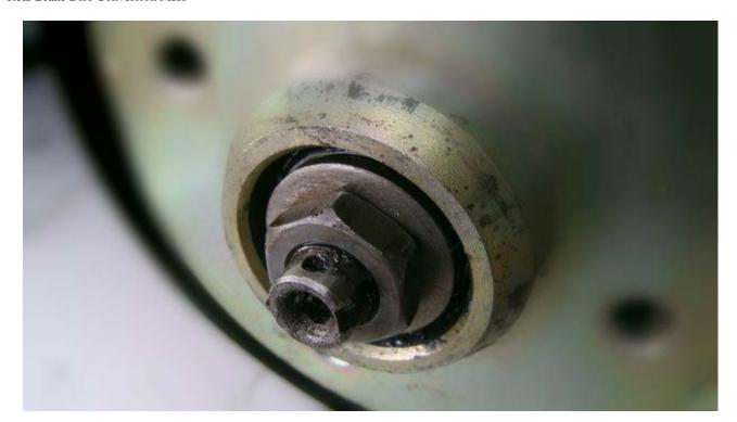
Then you can fit the locking cover over the nut. Make sure the nut is turned at an angle that leaves the small hole accessible on the end of the stub axle.
