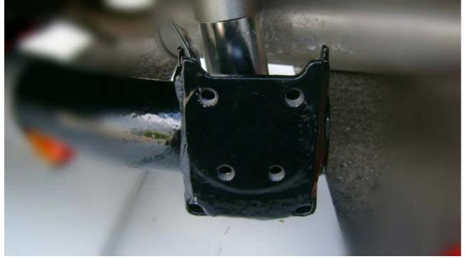
You will 1st be fitting the stub axle and dust cover (if fitting 1). The stub axle bolts are a 15mm. You will need to fit the stub axle with the carrier mounting holes closest to the rear side of the car. Only 1 of the stub axles will fit the way pictured due to the spacing of the bolts.
