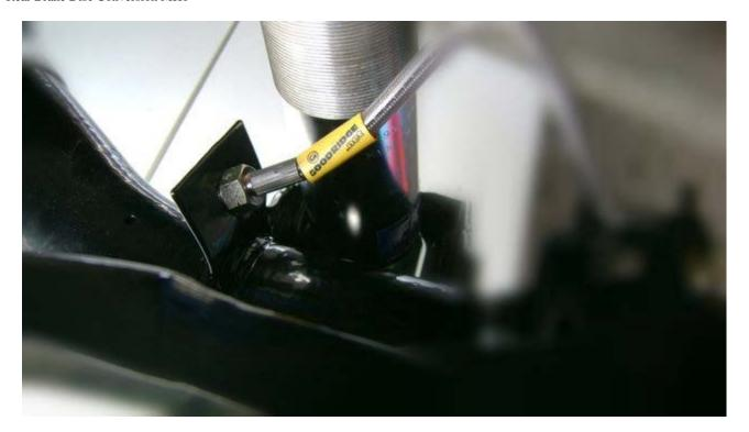
Now to put the handbrake cable on. sSlide it from under the axle and through the hole on the back of the
