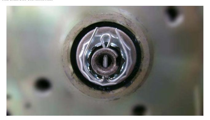
Now line the grease cap with grease and cover the end of the stub axle with grease. And tap the cap in to the end of the disk.
